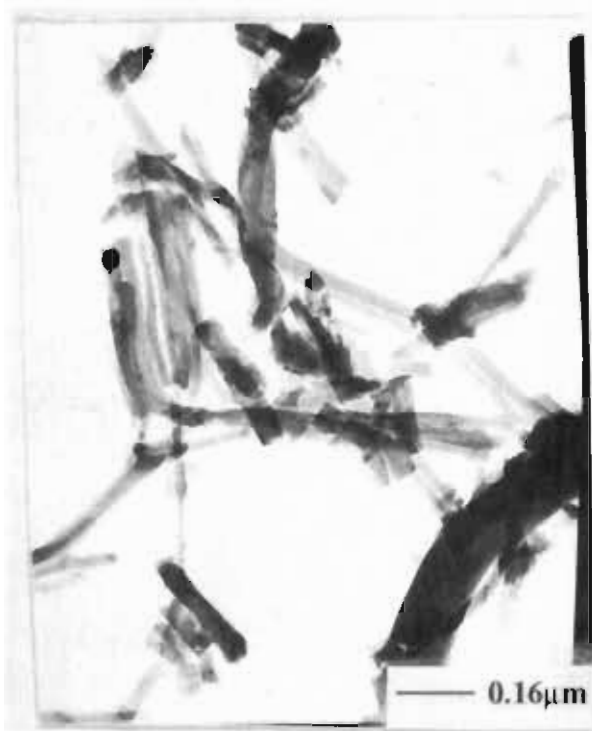
Figure 1. Transmission electron micrograph of the solid product formed upon reacting [EtZn(SBu^1)]_2 with H_2S at a flow rate of 5 cm^3/min in CH_2Cl_2 solution at 22 ^{\circ}C .
